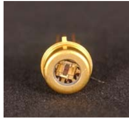
Figure 6. Optical channel monitor packaged in a TO-5 can.
